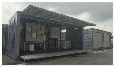
Alpha Biofuels also sets up micro-refineries for clients to convert waste cooking oil into biodiesel within their premises, such as this one at Asia Square Tower 2.
