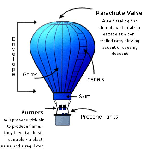
The burner uses propane gas to heat up the air in the envelope to move the balloon off the ground and into the air. The pilot must keep firing the burner at regular intervals throughout the flight to ensure that the balloon continues to be stable. Naturally, the hot air will not escape from the hole at the very bottom of the envelope as firstly, hot air rises and secondly, the buoyancy keeps it moving up.
