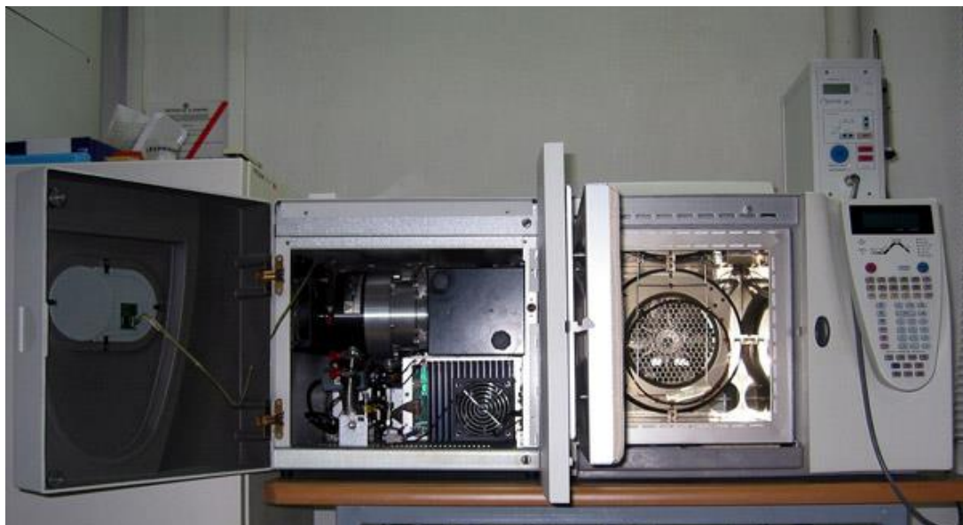
This Gas Chromatograph-Mass Spectrometer is similar to the one used in Zumberge's lab for separating, identifying and quantifying biomarkers in crude oils.
