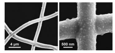
Adding a thin layer of metal onto plastic fibers helps bond together those points where they touch. Microscope images, above, show such a metal-plated mesh (with extreme close-up view at right).
