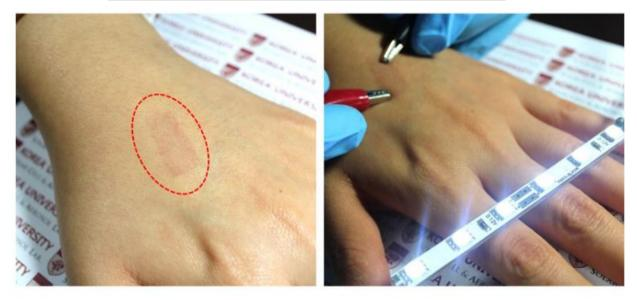
Flexible, see-through mesh of metal-covered plastic fibers (circled at left) conducts electricity and could be used in medical sensors as well as many electronic devices. Glowing LEDs (fingers at right) show the mesh is conducting electricity from the red and black clips on either side of the mesh.
